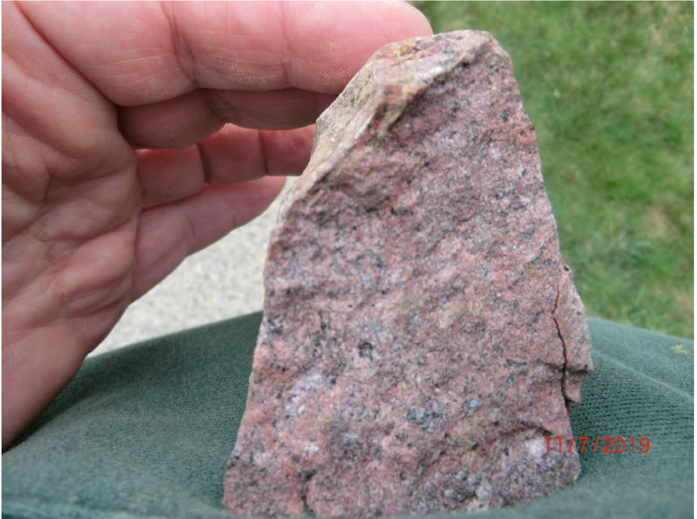
Figure 12 – Arkose bedrock encountered. Part of the Portland Arkose Formation.
